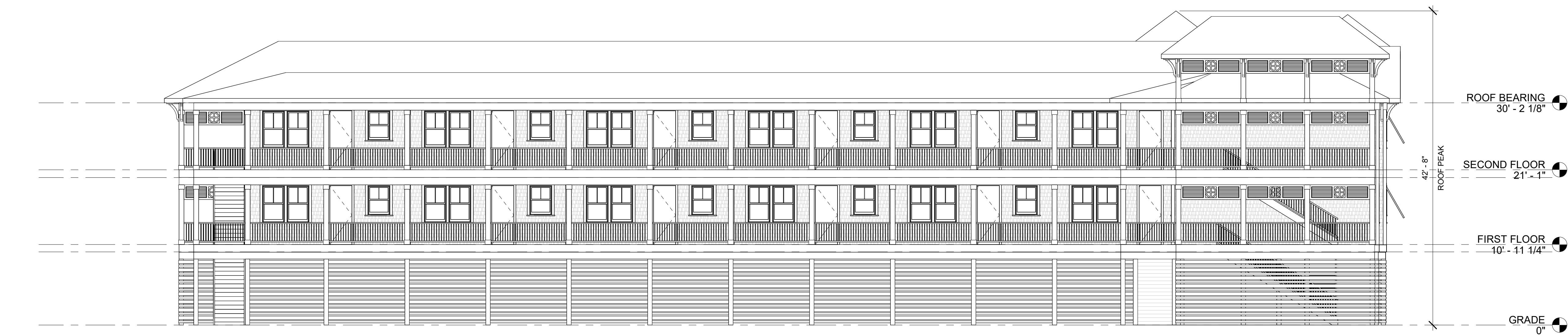
1 NORTH ELEVATION - ISLAND LIMOUSINE A2.2 1/8" = 1'-0"
